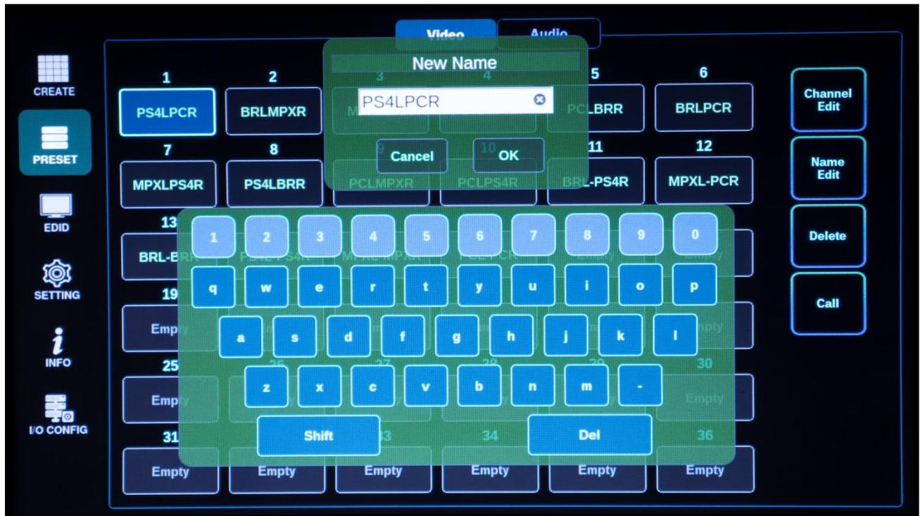
To edit the name of a preset, on the **PRESET** main menu, select the desired preset # and then press the **Name Edit** button. Users can name presets in a combination of letters and numbers using the keypad shown on the LCD. Press the **OK** button to save the name or **Cancel** to disregard the changes.
