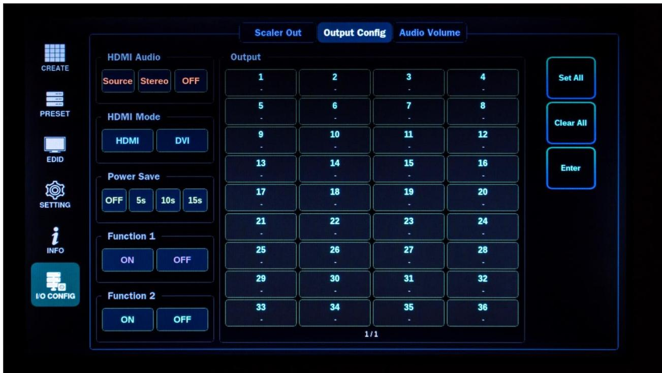
Configuration on each output of the Media Axis™ can be changed through the **Output Config** tab.
