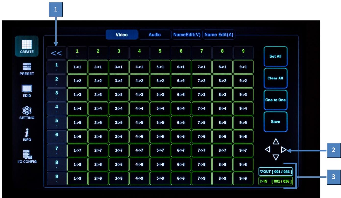
1. **Home Button** – press this button to go back to inputs 1 through 9 and outputs 1 through 9 no matter where you are in the inputs and outputs of the matrix
