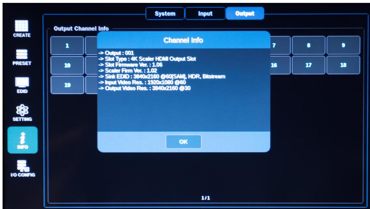
\*Output tab – press the desired output to check Channel Info
