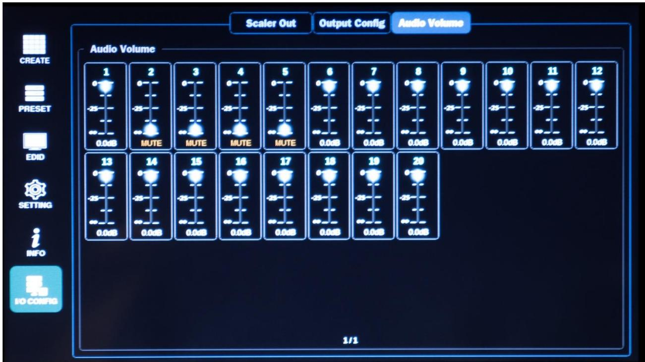
Media Axis™ allows users to change/mute audio volume for each individual output through the **Audio Volume** tab.
