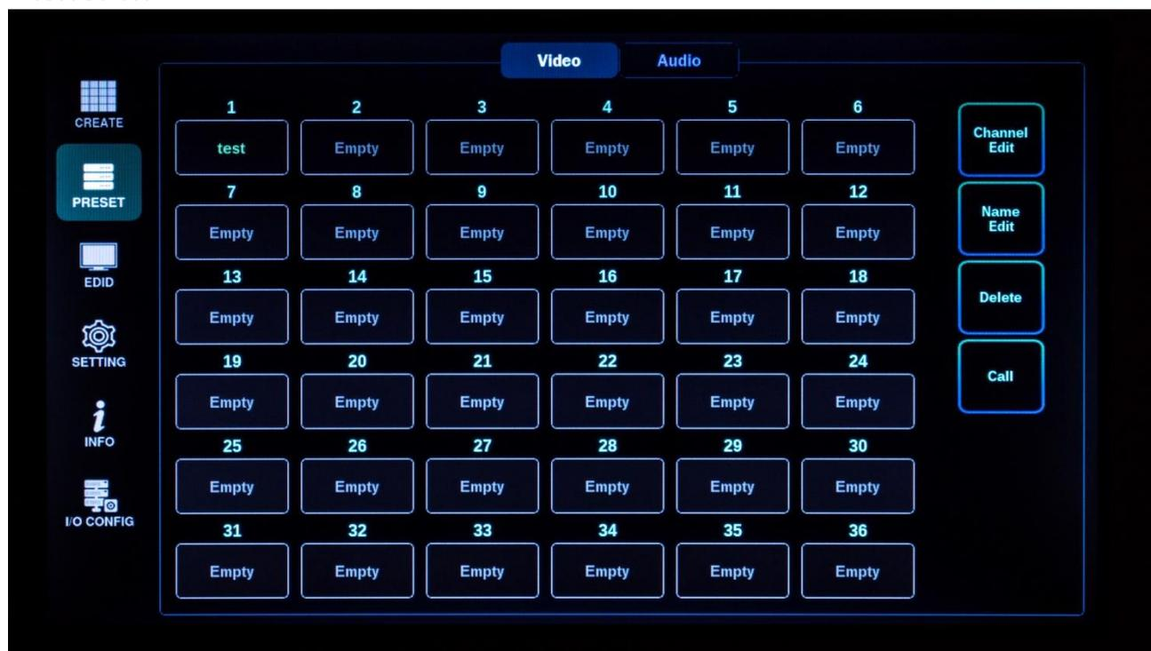
To create, edit channel, edit the name, delete, or recall, select the desired Preset number. The buttons on the righthand side have the following functions:
