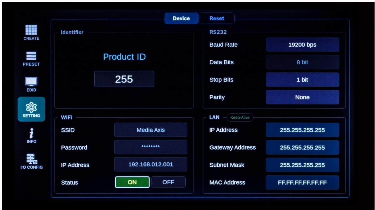
In the **Device** tab, there are four values that need to be set for serial communication: Baud Rate, Data Bits, Stop Bits, and Parity. Click and select each value using the touch screen and press the Enter button to save.
