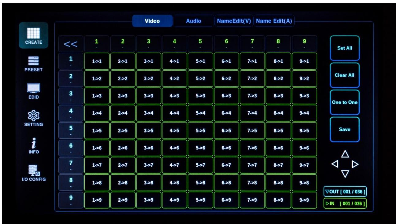
This section is to switch Video connections only. Select Input and Output numbers to route a source signal to destination devices. (for Example: select 2->1 = input 2 is routed to output 1)
