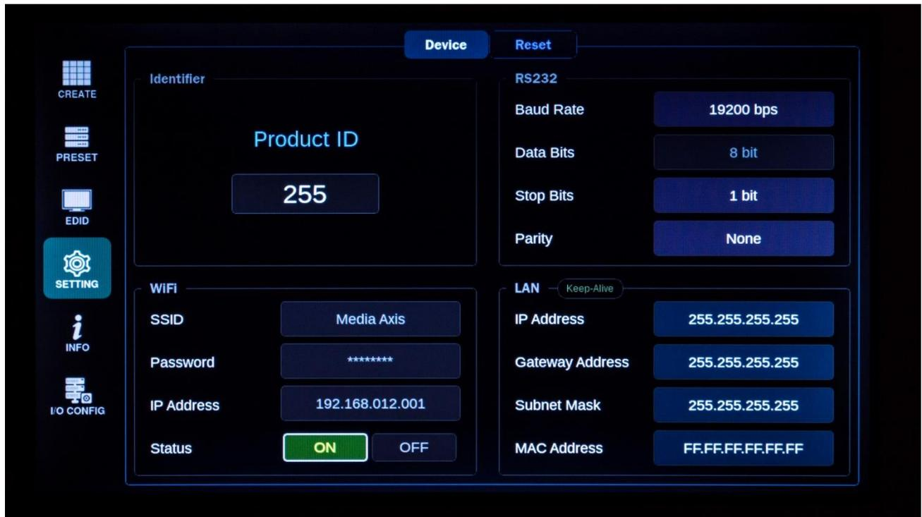
In the **Device** tab by setting different IDs to Media Axis™, up to 255 units of Media Axis™ Matrix Switchers can be connected and operated on the same network either via serial or LAN communication. The Product ID can be set between 001 ~ 255.
