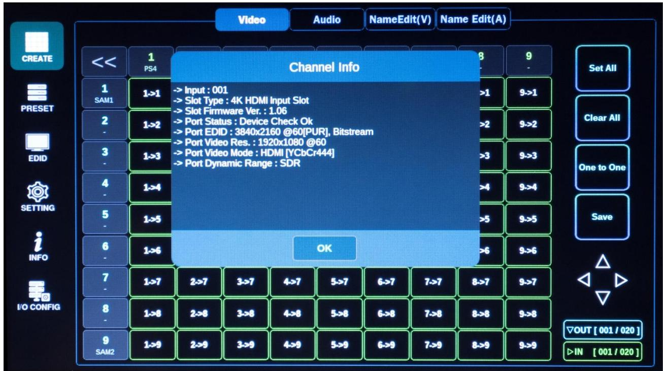
\*Horizontal #s are inputs and vertical #s are outputs
