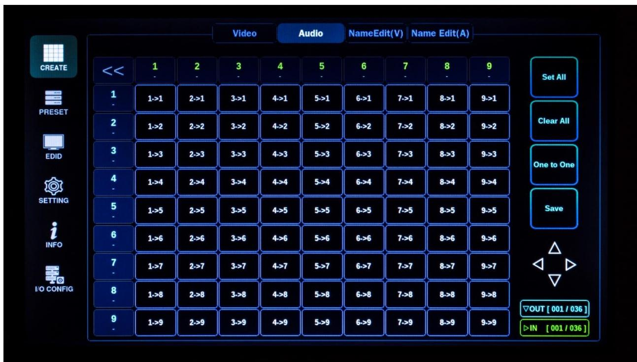
This section is to switch audio connections only. Select Input and Output numbers to route a source signal to destination devices. (for Example: select 2->1 = input 2 is routed to output 1)
