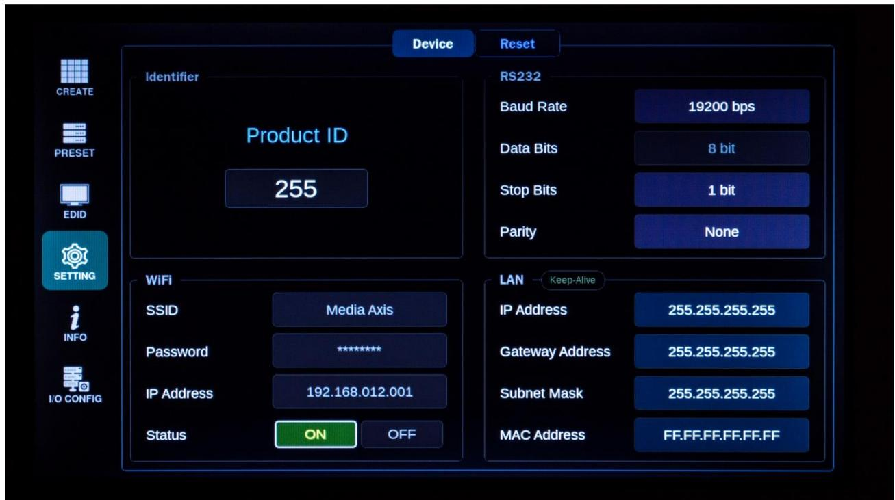
Media Axis™ can be controlled through the 10/100 base Ethernet port using either GUI (graphic user interfaces) or a command-line interface. The graphic user interfaces use a standard web browser such as Microsoft Internet Explorer.
